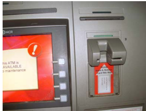
5. Card slot after Card reader attachment removed (ie: this is how the ATM should normally look)
