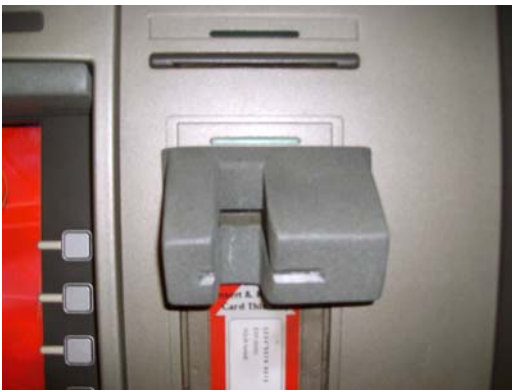
2. Close up of card reader attachment over card slot
